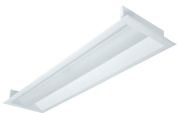
Overall dimensions including flange: 14" x 50" Required ceiling opening: 12 1/2" x 48 1/2"
