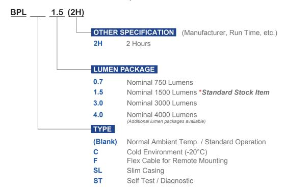
Emergency Lighting Control Device for Generator or Central Inverter Supplied Power
