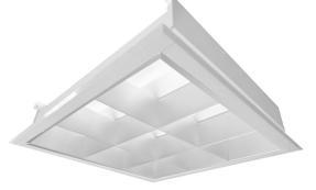
Overall dimensions including flange: 26" x 26" Required ceiling opening: 24 1/2 " x 24 1/2"
