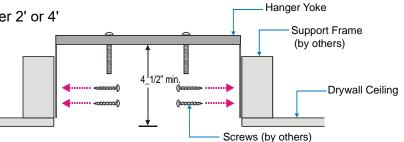
2). There are four 3/8" diameter pre-punched knockouts on back side of fixture housing for hanger yokes. Remove the four knockouts.
