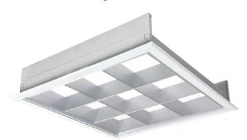
Overall dimensions including flange: 26" x 26" Required ceiling opening: 24 1/2 " x 24 1/2"
